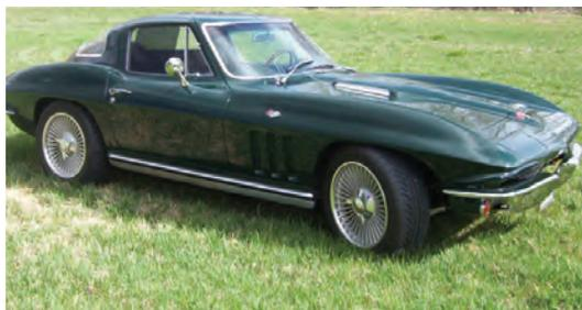
This was the last Corvette that Dick Guldstrand built. In 2009 Victoria Hearst discussed having an older body-style Corvette built on a newer frame. A 1965 was placed on a C4 frame from Newman Car Creations and was fitted with an LS1 engine. Guldstrand massaged the 346 ci. V8 to 400 hp and installed a four-speed automatic transmission since Hearst couldn't drive a stick. A good bit of fabrication and custom work went into this build.
